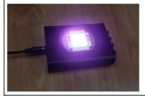
Size(mm):20 x 80 x 30Weight:230 gPower:24V, 3ARange (m):Up to 25FOV:120 degreesConnects to Basaltdriver board
