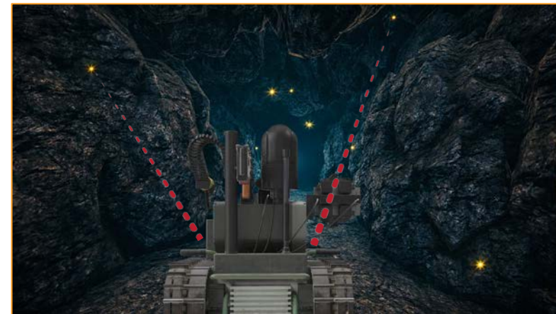
Autonomous navigation: In large indoor facilities and tunnels using installed light sources
